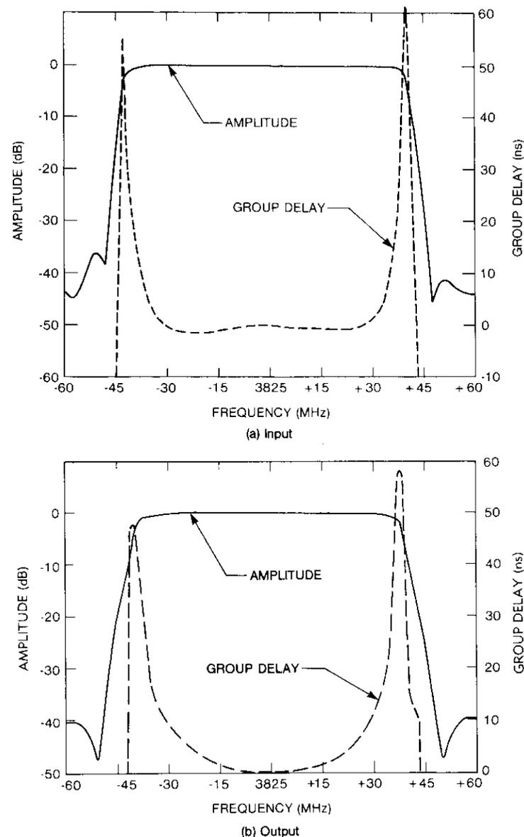
Figure 34. Channel 3-4 Transponder Input and Output Filters Amplitude and Group Delay Responses
