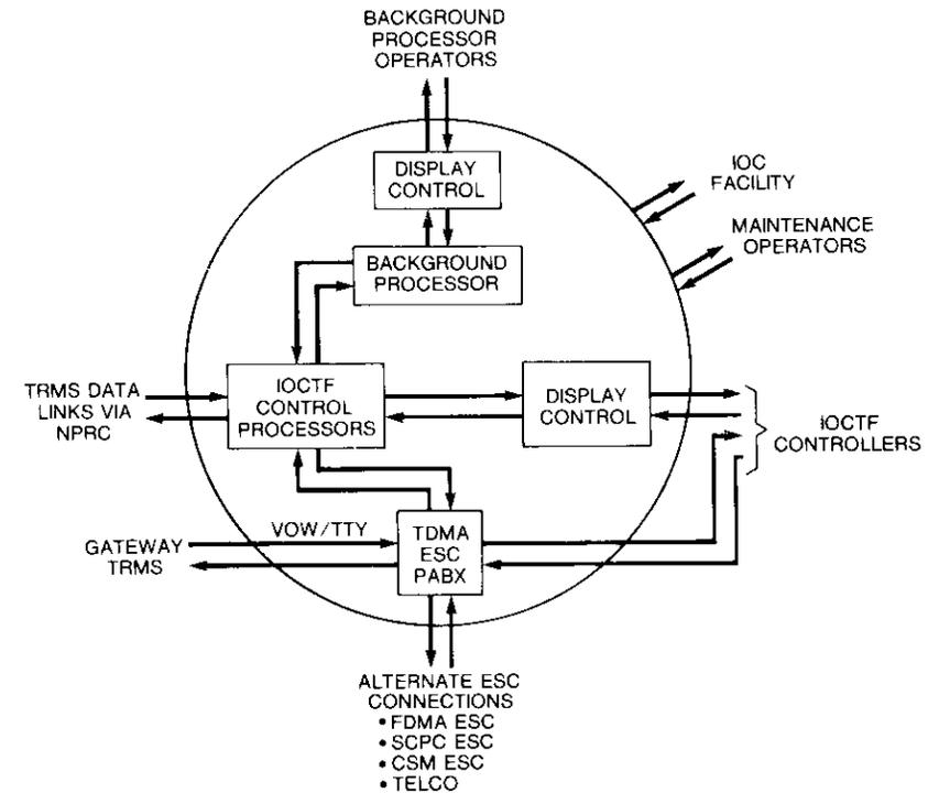
Figure 3. IOCTF External Interfaces
