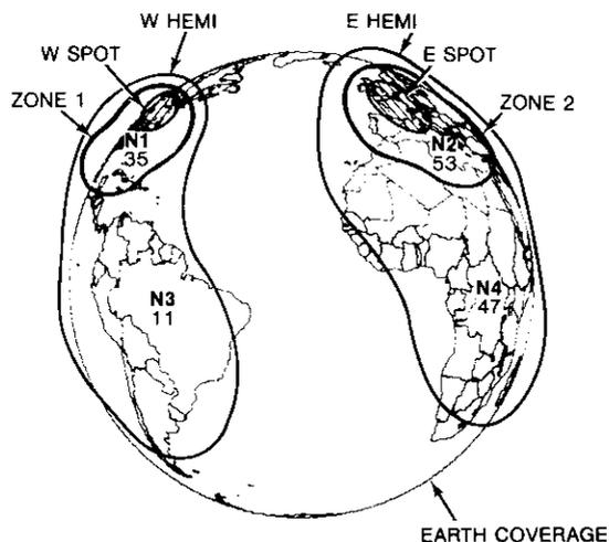
Figure 1. INTELSAT V AOR Beam Coverages
