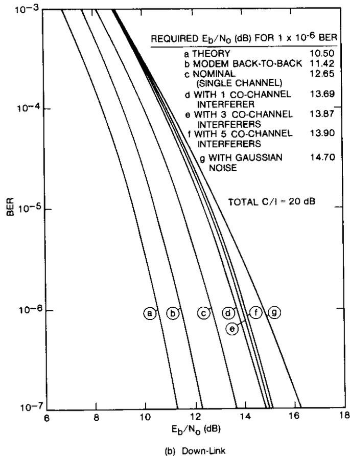
Figure 22b. Additional Computer Simulation of CCI Performance (Continued)
