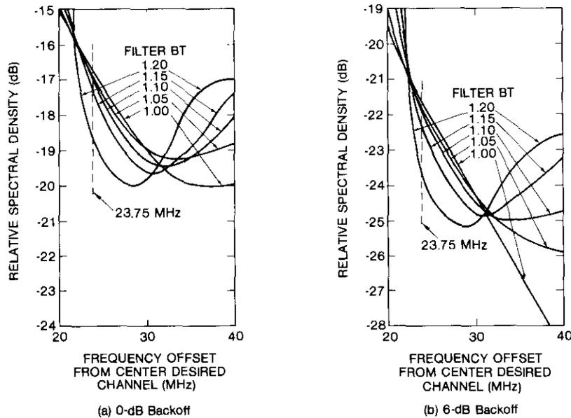
Figure 11. Summarized HPA Regrowth Spectra for Filtered QPSK (filter A, 30-percent Nyquist)
