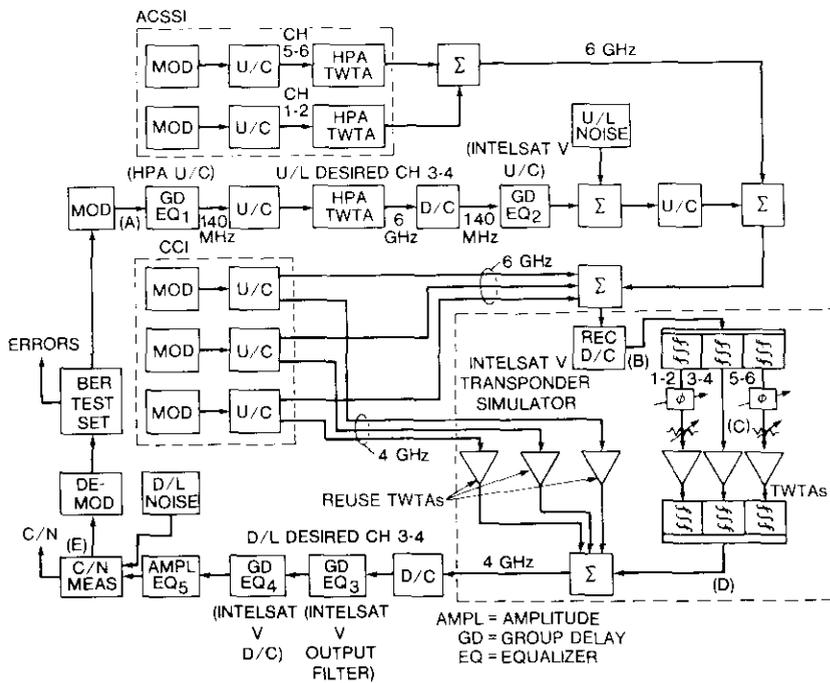
Figure 14. Simplified Block Diagram of the INTELSAT V Hardware Simulation Experiment
