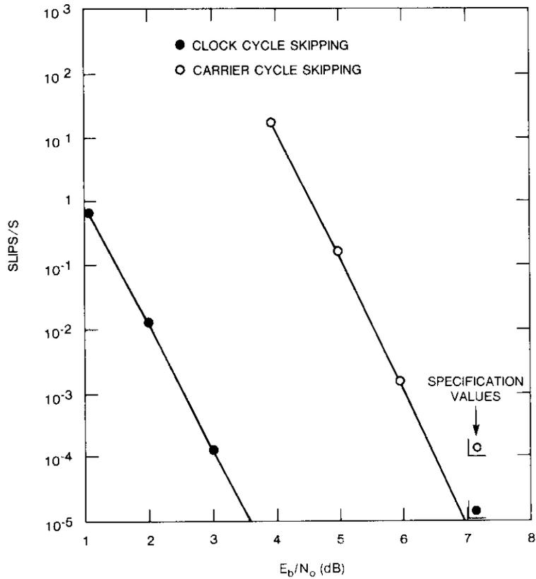
Figure 5. Carrier and Clock Cycle Slipping vs  $E_b/N_0$
