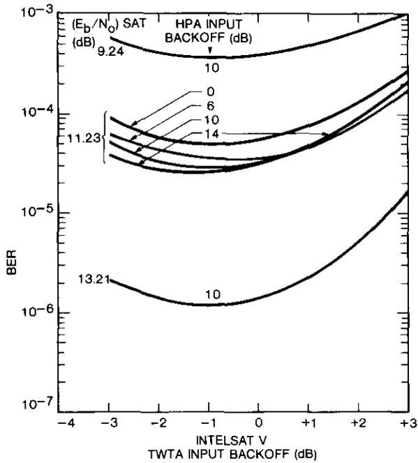
Figure 19. Channel 3-4 Performance as a Function of HPA and INTELSAT V TWTA Input Backoffs
