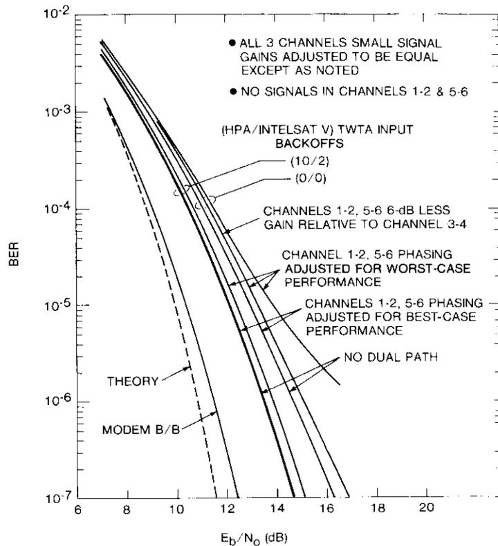
Figure 32. INTELSAT V Channel 3-4 Performance With Channel 1-2 and Channel 5-6 DPI Effects
