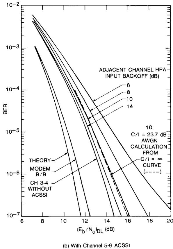
Figure 30b. *INTELSAT V Channel 3-4 10/2 Performance With Up-Link ACSSl (Continued)*
