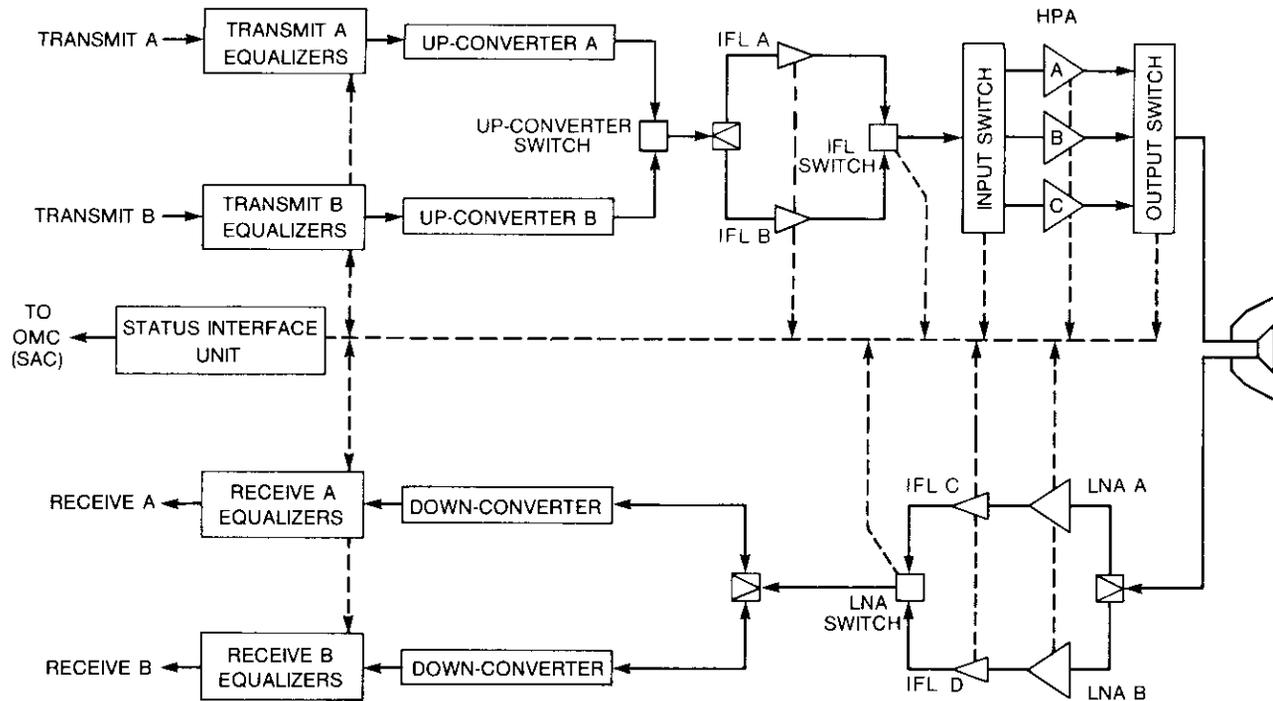
Figure 3. TDMA Traffic Terminal IF/RF Equipment
