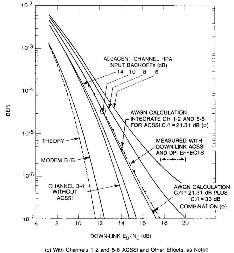
Figure 30c. *INTELSAT V Channel 3-4 10/2 Performance With Up-Link ACSSl (Continued)*
