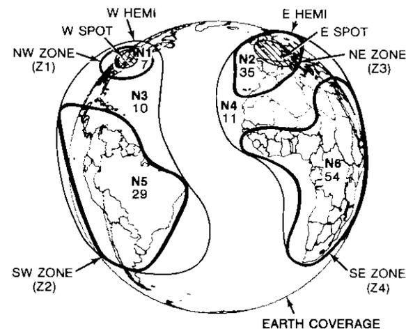
Figure 4. INTELSAT VI AOR Beam Coverages
