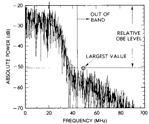
Figure 13. Computer Simulation of Spectrum of Type I Modem Filters With HPA Input Backoff of 12 dB
