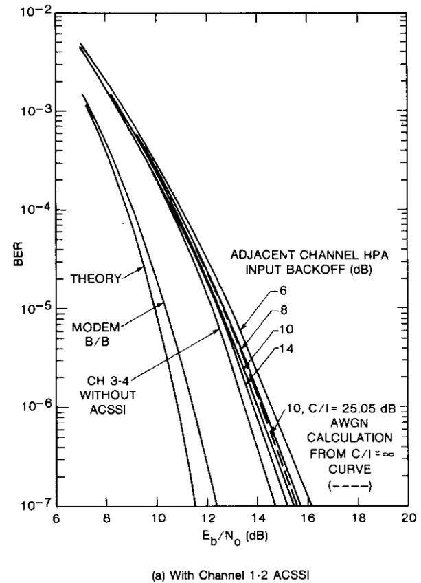
Figure 30a. INTELSAT V Channel 3-4 10/2 Performance With Up-Link ACSSI
