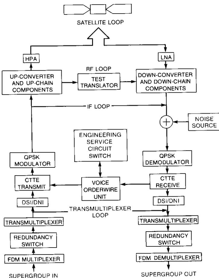
Figure 1. Loop Test Configurations
