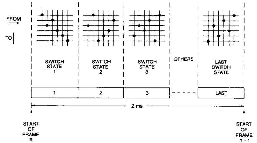
Figure 8. Typical Switch-State Time Plan For  $6 \times 6$  Beams
