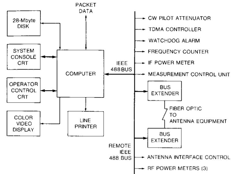
Figure A-1. TSM Processor Subsystem Block Diagram
