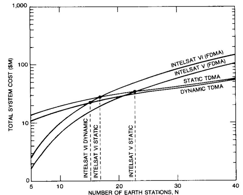
Figure 9. Earth Station Costs vs Number of Stations for One Satellite
