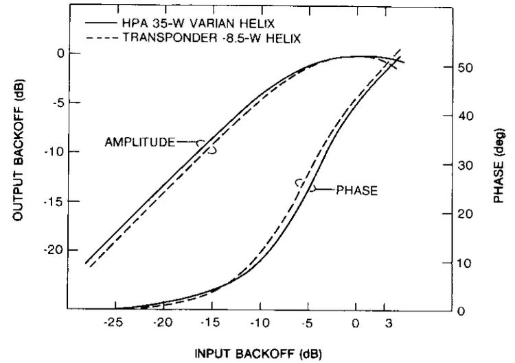
Figure 17. Desired Channel 3-4 TWAs Single-Carrier Characteristics
