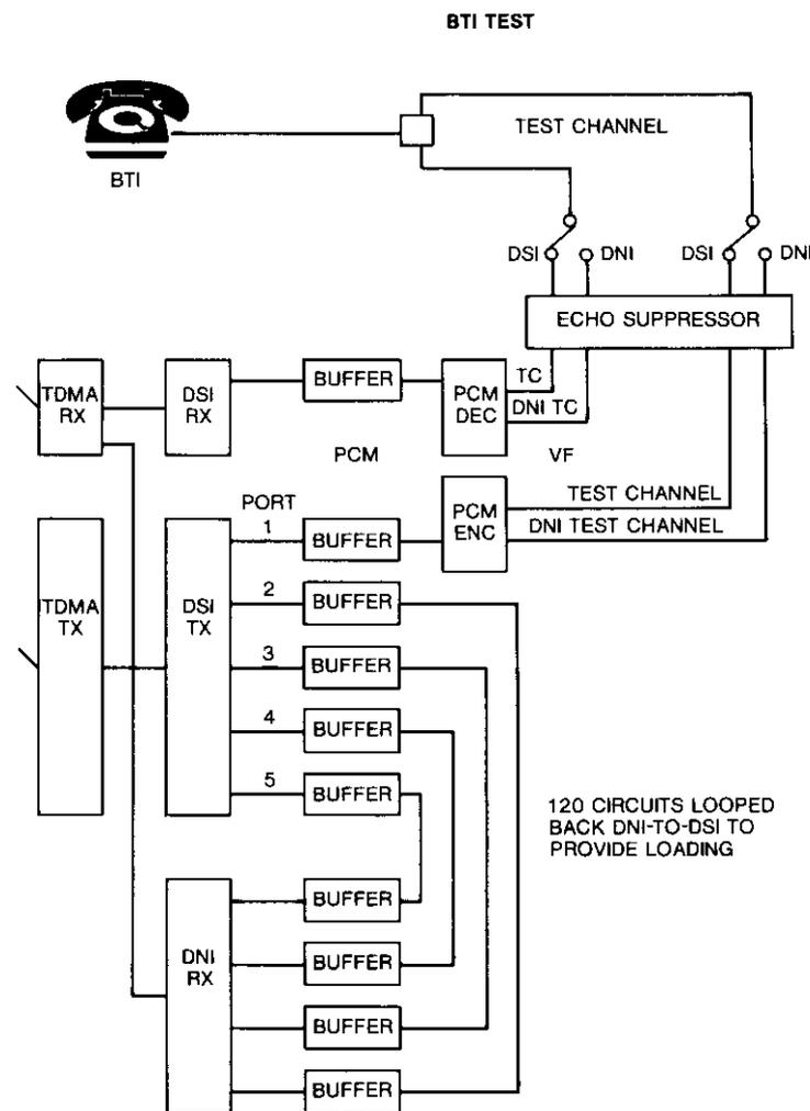
Figure 2. U.K. Circuit Configuration
