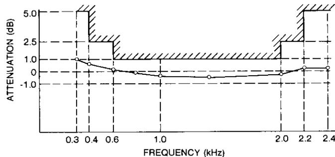
Figure 9. Delta Codec Frequency Response
