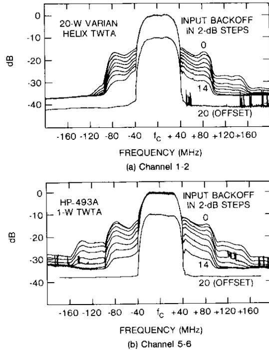
Figure 29. Adjacent Channel Signal Spectra Showing Sideband Regrowth
