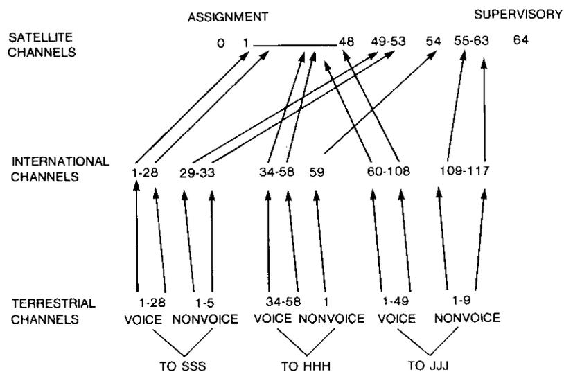
Figure 6. Channel Numbering on DSI Multidestination Sub-Burst From Station AAA to Stations SSS, HHH, and JJJ
