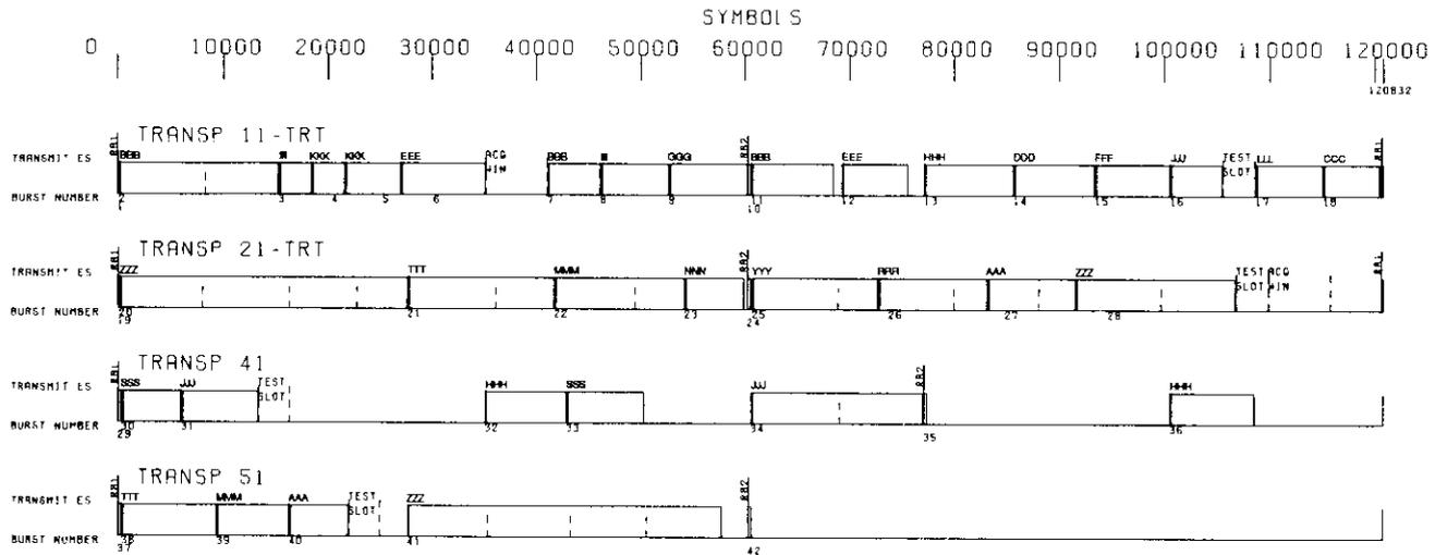
Figure 5. Sample Plot of TDMA Burst Schedule
