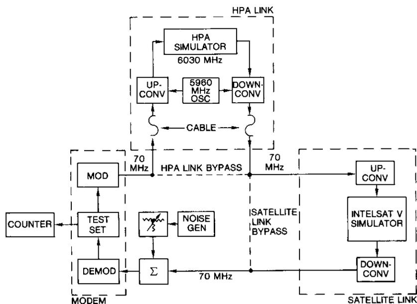
Figure 3. 60-Mbit/s QPSK INTELSAT IV Transmission Test Configuration Functional Block Diagram
