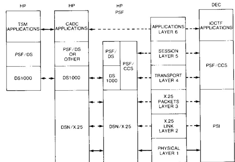
Figure 5. Communications Software Protocol Layers
