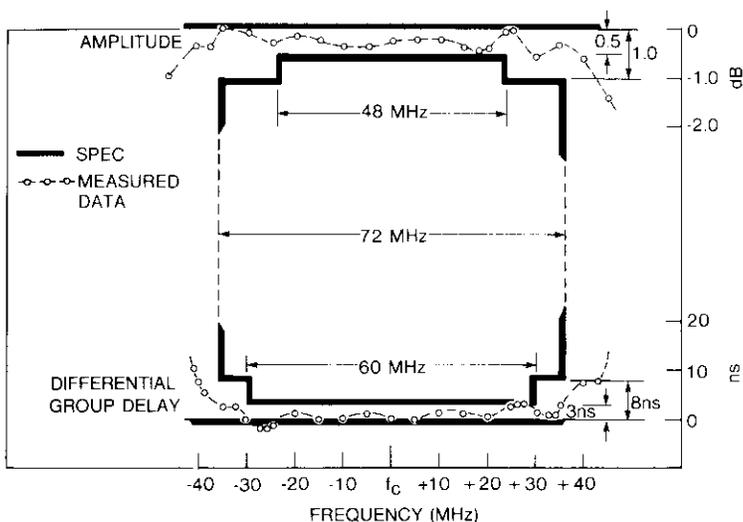
Figure 35. Channel 3-4 Down-Link Amplitude and Group Delay Responses
