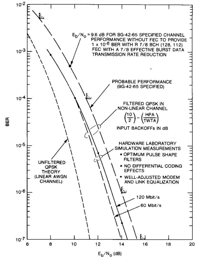
Figure 2. QPSK Modem Performance in the Nonlinear Channel
