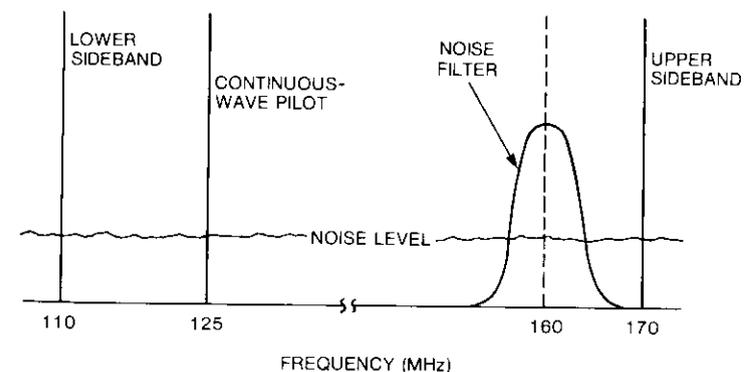
Figure 4. IF Spectrum During Carrier and Bit Timing Recovery
