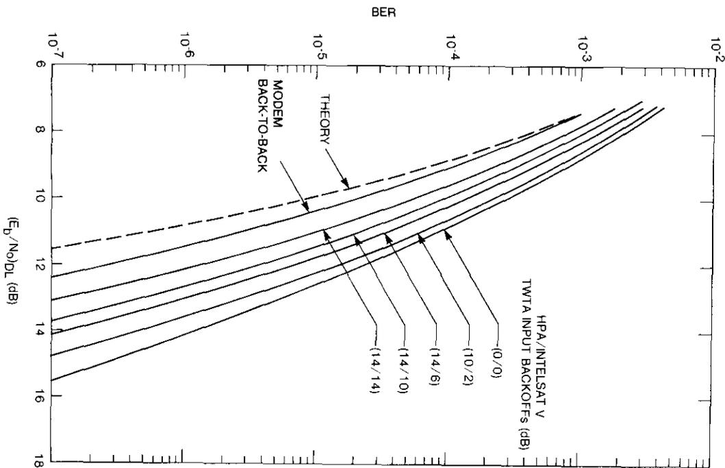
Figure 15. 120-Mbit/s QPSK Modem Filter Type III Performance in INTELSAT V Channel 3-4 Without Interference
