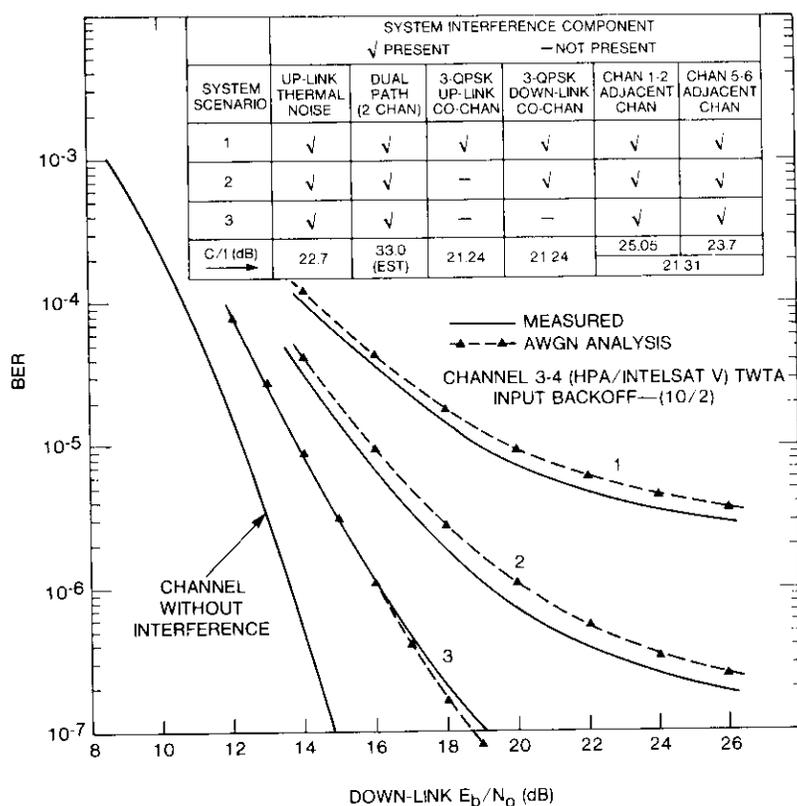
Figure 38. Channel 3-4 Static BER Performance With Three Multiple Interference Scenarios
