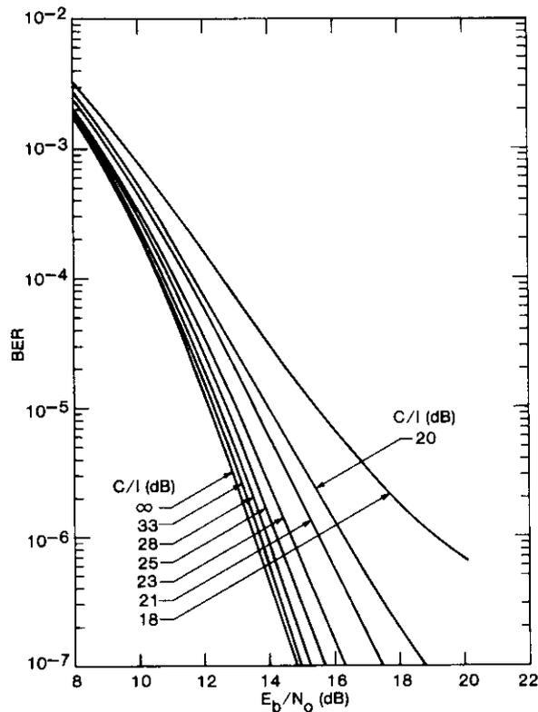
Figure 31. *Modem In-Channel Performance Variation With AWGN Interference Calculation as a Function of C/I*
