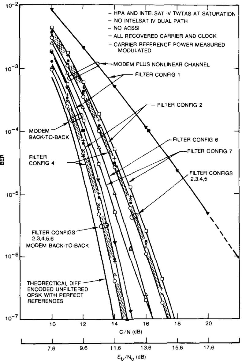
Figure 5. BER Performance for 60-Mbit/s QPSK Modem Filter Hardware Study
