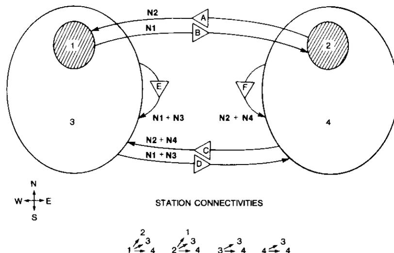
Figure 3. INTELSAT V Beam Cells and Minimum Connectivities
