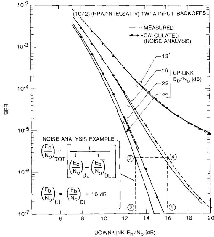
Figure 24. Performance Impairment Due to Up-Link Thermal Noise
