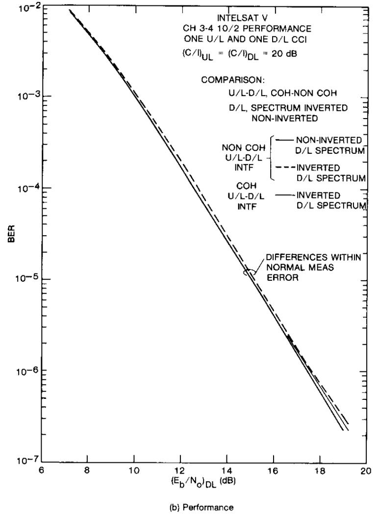
Figure 23b. Initial Investigation of Simultaneous Single Up-Link and Down-Link CCI Hardware Simulation (Continued)
