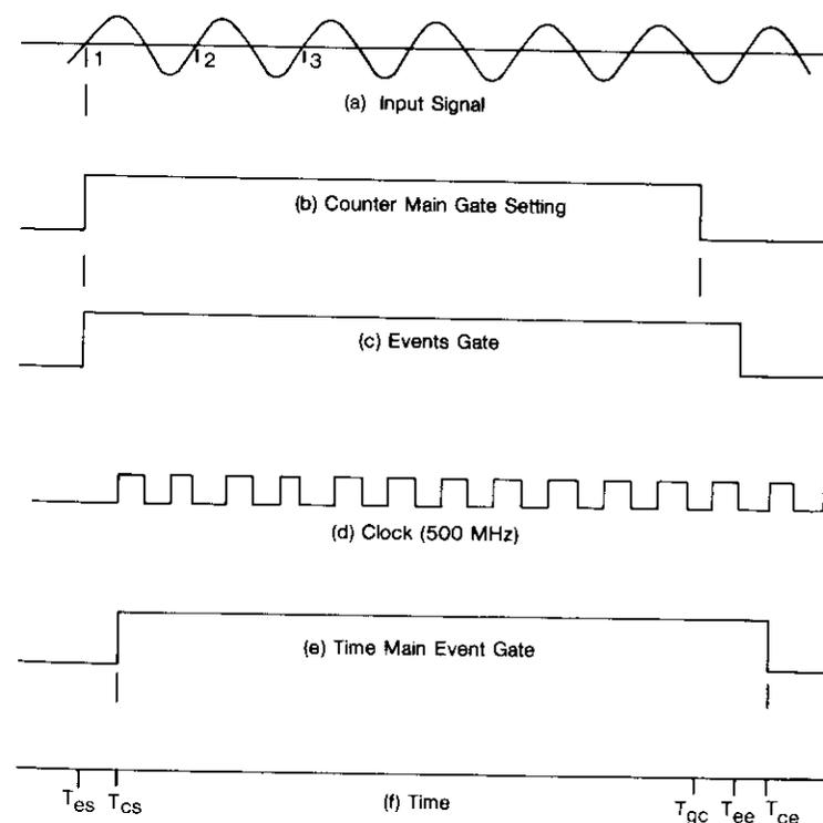
Figure 5. TSM Counter Measurement Timing
