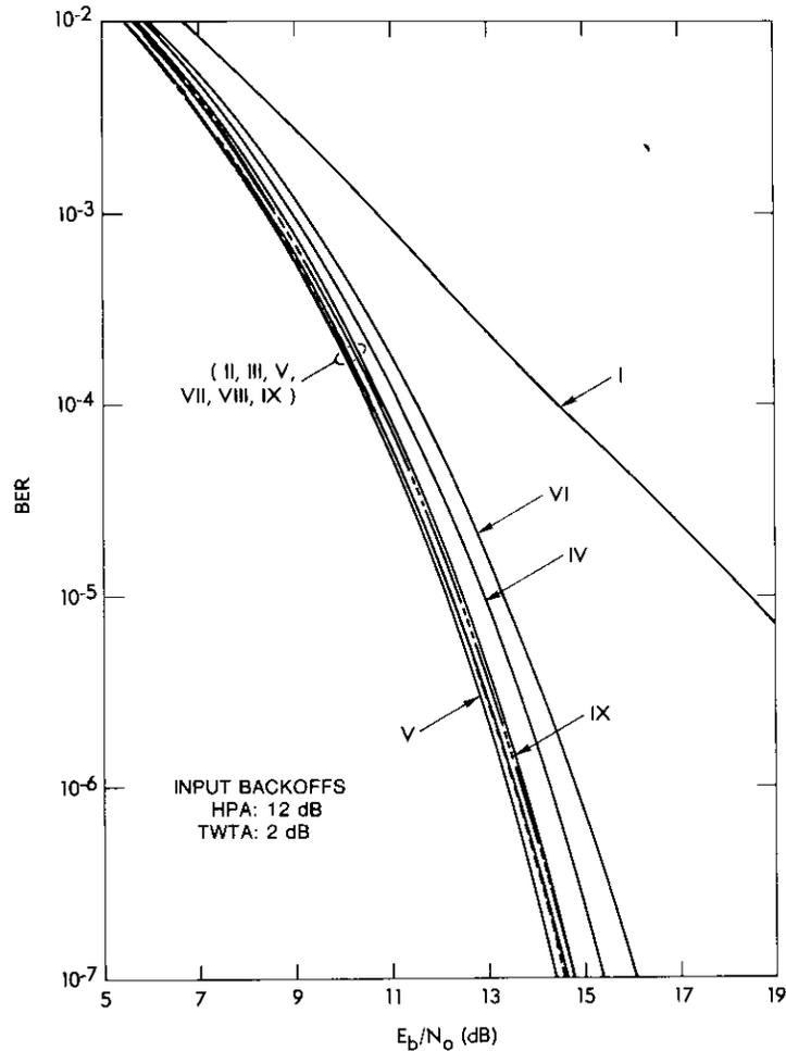
Figure 7. BER Performance for Computer Simulation Modem Filter Study
