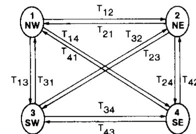
Figure 10. Traffic Coefficients For a Four-Beam Network
