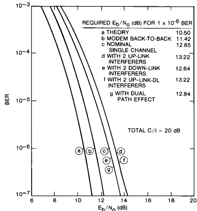
Figure 28. Computer Simulation of ACSSI and DPI Effects
