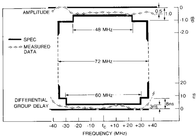
Figure 33. Channel 3-4 Up-Link Amplitude and Group Delay Responses
