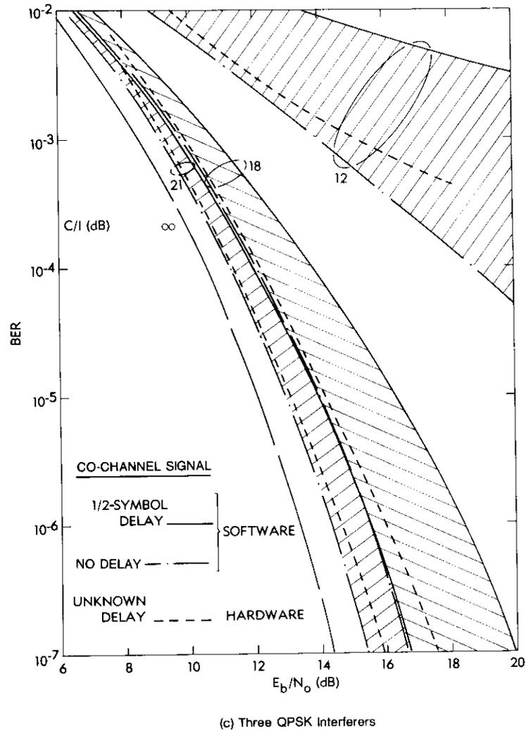
Figure 21c. Hardware/Software BER Performance Comparisons of Satellite System With Up-Link CCI (Continued)
