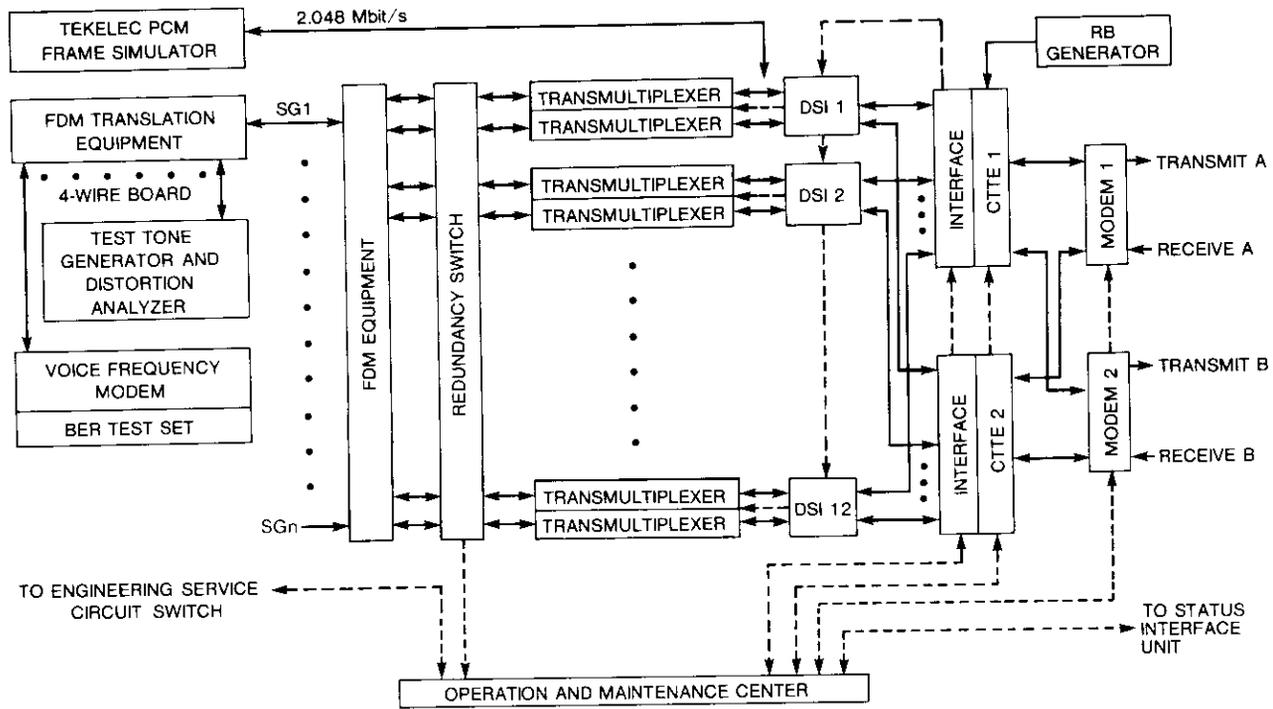
Figure 2. TDMA Traffic Terminal Baseband Equipment
