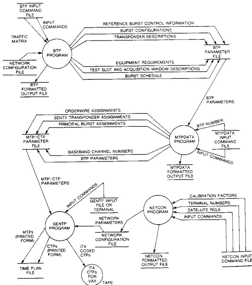
Figure 8. BTP/MTP/CTP Software System Data Flow
