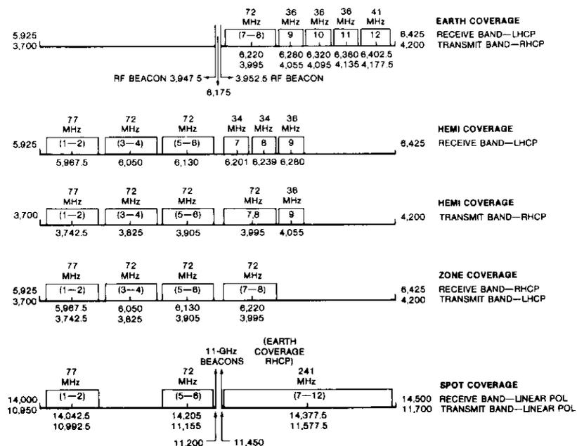
Figure 2. INTELSAT V Transponder Frequency Plan
