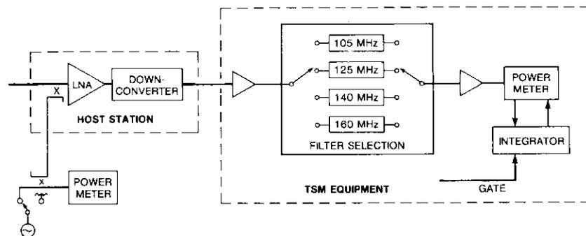
Figure 3. Simplified Gain and Power Measurement Block Diagram
