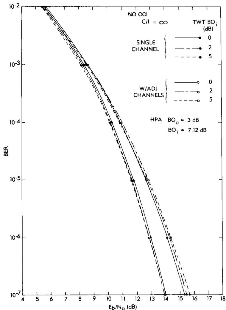
Figure 27. Computer Simulation of INTELSAT V With and Without Two-Channel ACSSI
