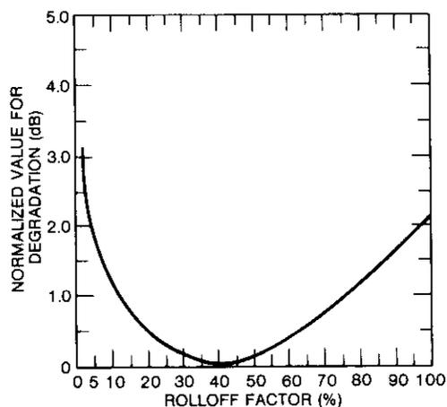
Figure 8. Filter Type III Nonlinear Channel Impairment vs Filter Rolloff Factor
