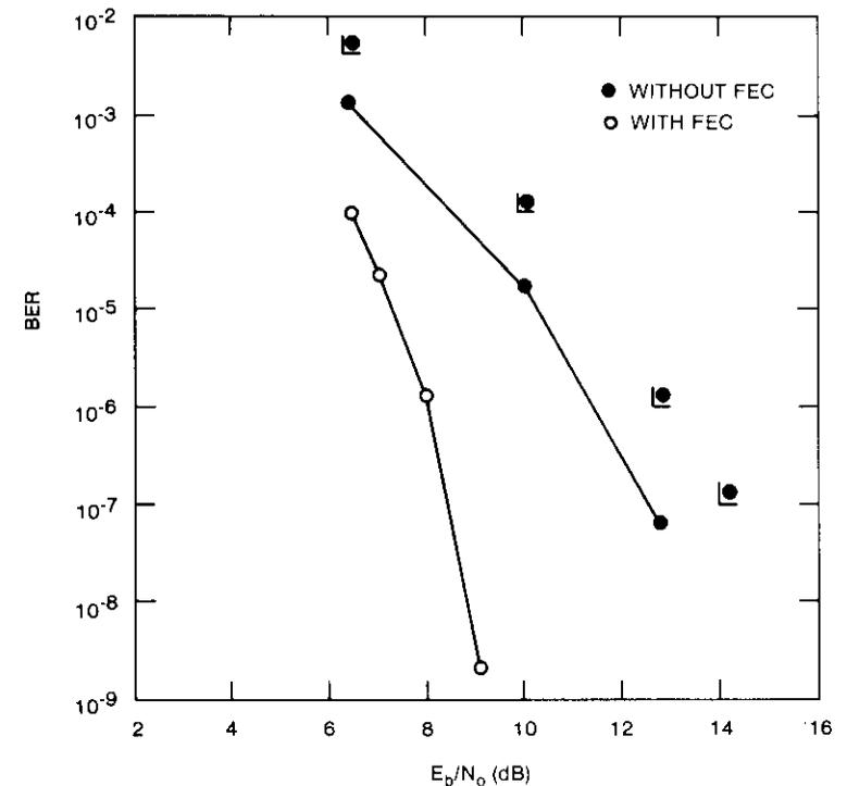
Figure 10. DSI Channel BER Performance (IF loop with DSI loading)
