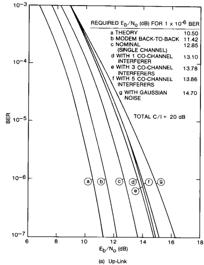
Figure 22a. Additional Computer Simulation of CCI Performance
