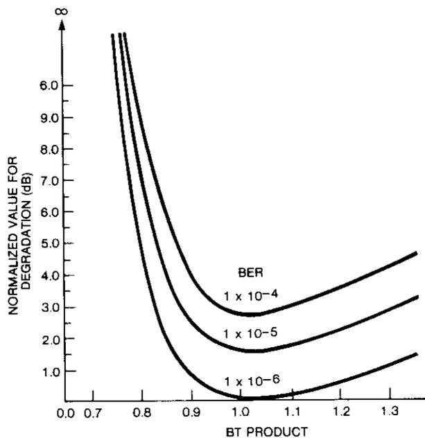
Figure 9. Filter Type III Nonlinear Channel Impairment as a Function of Receiver Filter BT Product
